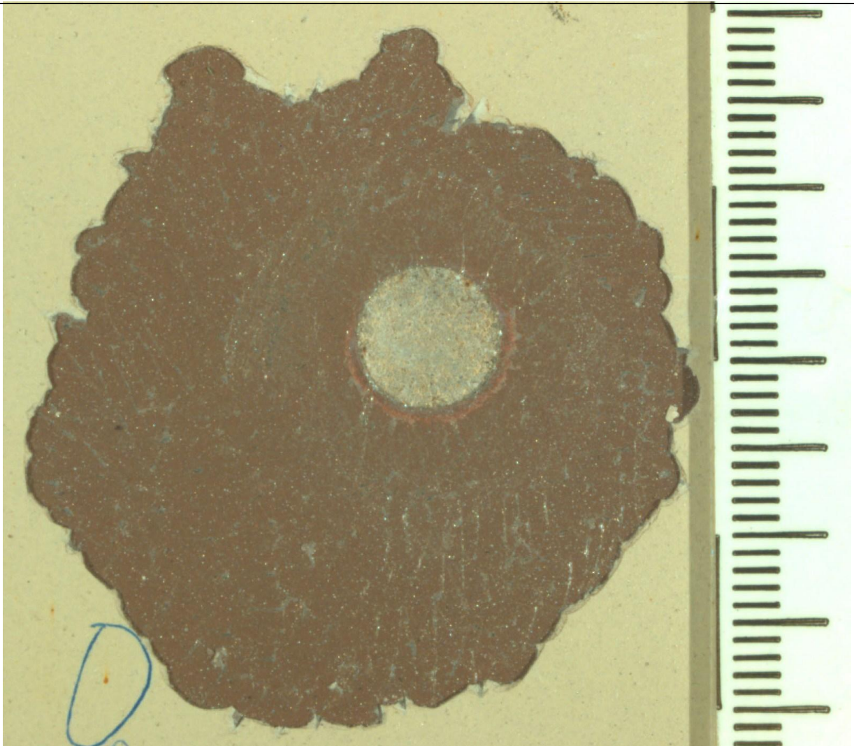
Figure C-7 Disbonding from artificial holiday, bottom wave tank panel (example picture not connected to example results in this model report).
